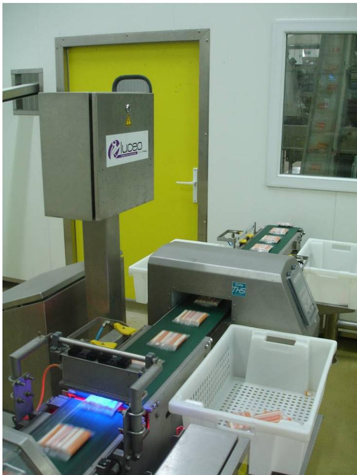
An inspection station installed between the flow packing machine and the pasteurisation tunnel
